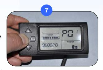
P0 2 (photo 8): the motor rotate one cycle, the number of sampling signal by display.
