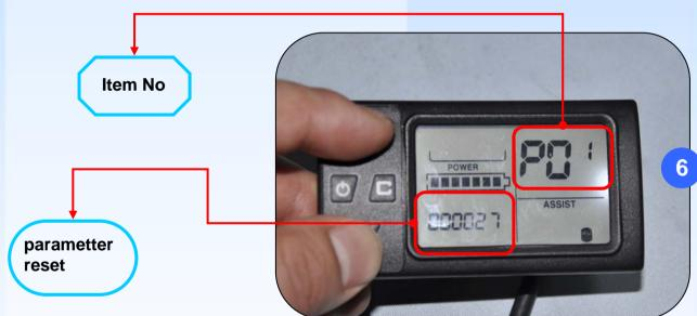
The parameter which can be reset containing wheel size(inch), numbers of magnetic jar, LCD screen light, undervoltage value and so on. Enter to the setup page:
