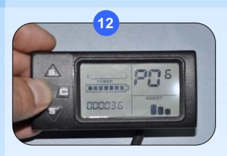
P0 6 (photo 12): setup the working voltage of battery: 24V, 36V, 48V. The reset working voltage should be same as the actural battery capacity. Otherwise the all system will not work.
