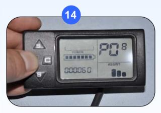
P0 8 (photo 14): setup the phase of motor; it is just available with the brushless motor, the setting value is according to different motor type, if setup at 60 means 60° overlap angle, If setup at 120 means 120° overlap angle. The setting value should be same as motor phase.
