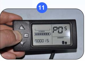
P0 5 (photo 11): setting of the max electric current of controller. The upper limit should be decided by the maximum current of controller. If the normal maximum current of controller is 15A, then the setting scope is 1-15A, can not be more than 15A, otherwise may break the controller.
